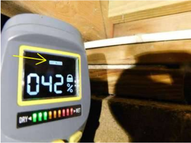
Photo 26-5 The meter is set to, "Softwood" as indicated by the yellow arrow. For wood, moisture is excessive when it reaches the mid 20% range. 42% is excessive as confirmed by the light bar again: Lit to the red.
