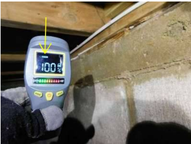
Photo 26-3 With the moisture meter set to, "Masonry" as indicated by the yellow arrow. The concrete block is holding 100% moisture. Notice the light-bar too: Green to yellow to red lights.
